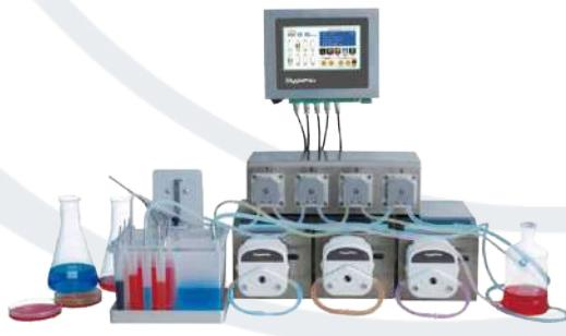
Application 2: PDSIV. One controller with 7 pump units, 4 HF-MiniPump and 3 HF-YZ1515x pump heads, for different liquid filling with different time sequence.
