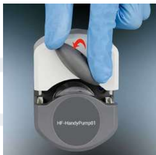
1. Turn the knob anticlockwise 180°, open the upper block.
