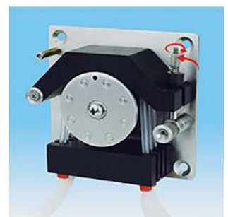
4. Turn spanner anticlockwise, locking the upper block, micro adjust the occlusion.
