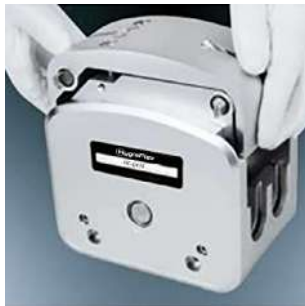
1. Lift both side levers, take off the upper block.
