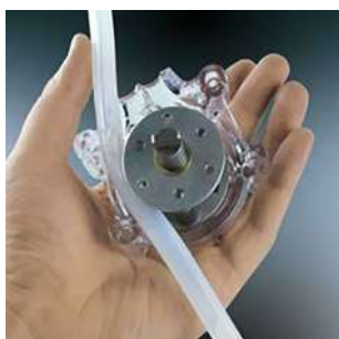
A. Disassemble the pump head and press the tubing on the rollers.
