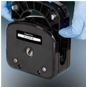
1. Lift both side levers, take off the cartridge or upper block.
