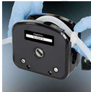
2. Put the tubing with cartridge or connector into pump housing.
