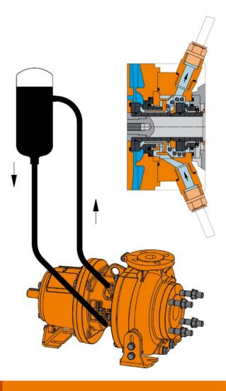
Pump with thermosyphon vessel
