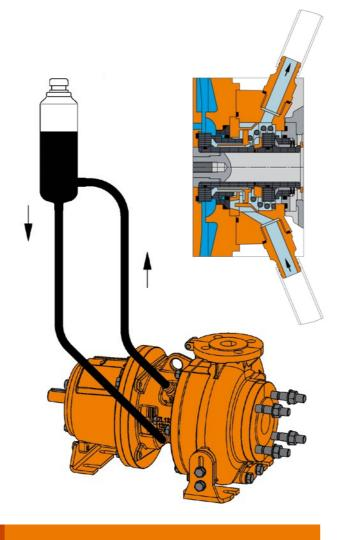
Pump with quench tank
