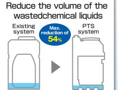
The volume of the wasted chemical liquids is reduced by incorporating shapes for the bottom of the tank and for the suction valve position, etc. that minimize the level of the chemical liquids remaining.
