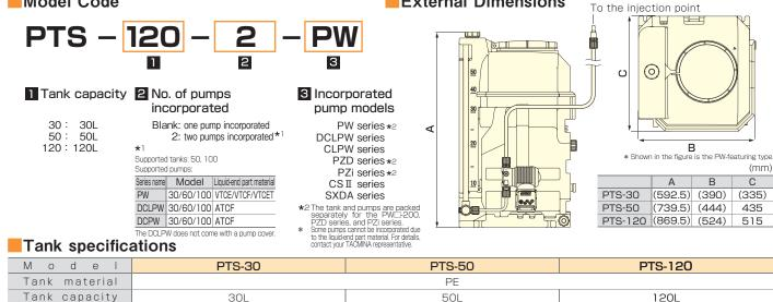
Weight (tank only) 4 kg 9 kg \*Install a shade or other type of awning since exposure to direct sunlight or ultraviolet rays may cause discoloration and/or deterioration.
