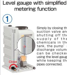
Simply by closing the suction valve and shutting off the supply of the chemicals in the tank, the pump's discharge volume can be checked using the level gauge while keeping the pipes connected.
