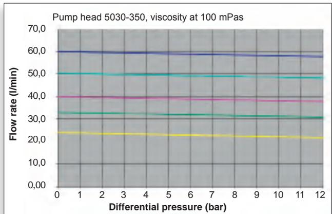
1725 RPM | 1450 RPM | 1150 RPM | 950 RPM | 690 RPM
