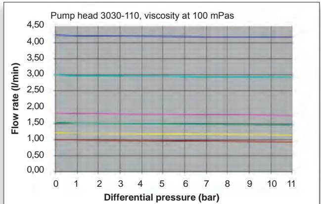
4000 RPM | 2830 RPM | 1725 RPM | 1450 RPM | 1150 RPM | 950 RPM
