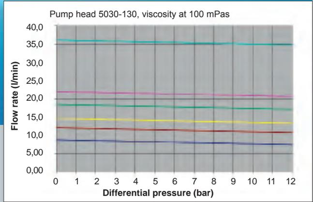
2830 RPM | 1725 RPM | 1450 RPM | 1150 RPM | 950 RPM | 690 RPM
